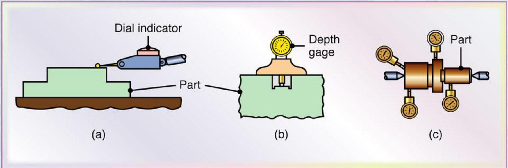
Figure 35.4 Three uses of dial indicators: (a) roundness, (b) depth, and (c) multiple-dimension gaging of a part.
