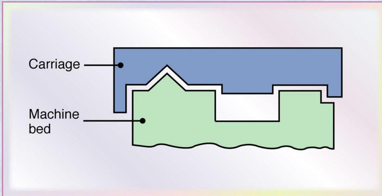
Figure 35.1 Cross-section of a machine-tool slideway. The width, depth, angles, and other dimensions all must be produced and measured accurately for the machine tool to function as expected.
