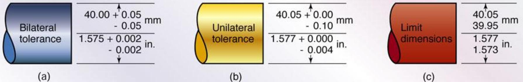
Figure 35.18 Various methods of assigning tolerances on a shaft: (a) bilateral tolerance, (b) unilateral tolerance, and (c) limit dimensions.
