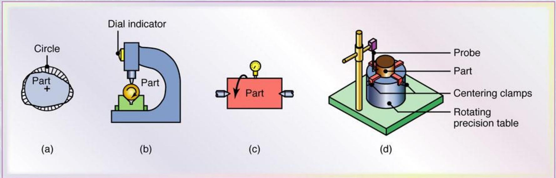
Figure 35.7 (a) Schematic illustration of out-of-roundness (exaggerated). Measuring roundness using (b) a V-block and dial indicator, (c) a round part supported on centers and rotated, and (d) circular tracing. *Source:* After F. T. Farago.
