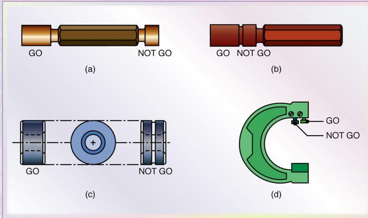
Figure 35.10 (a) Plug gage for holes with GO and NOT GO on opposite ends. (b) Plug gage with GO and NOT GO on one end. (c) Plain ring gages for gaging round rods. Note the difference in knurled surfaces to identify the two gages. (d) Snap gage with adjustable anvils.
