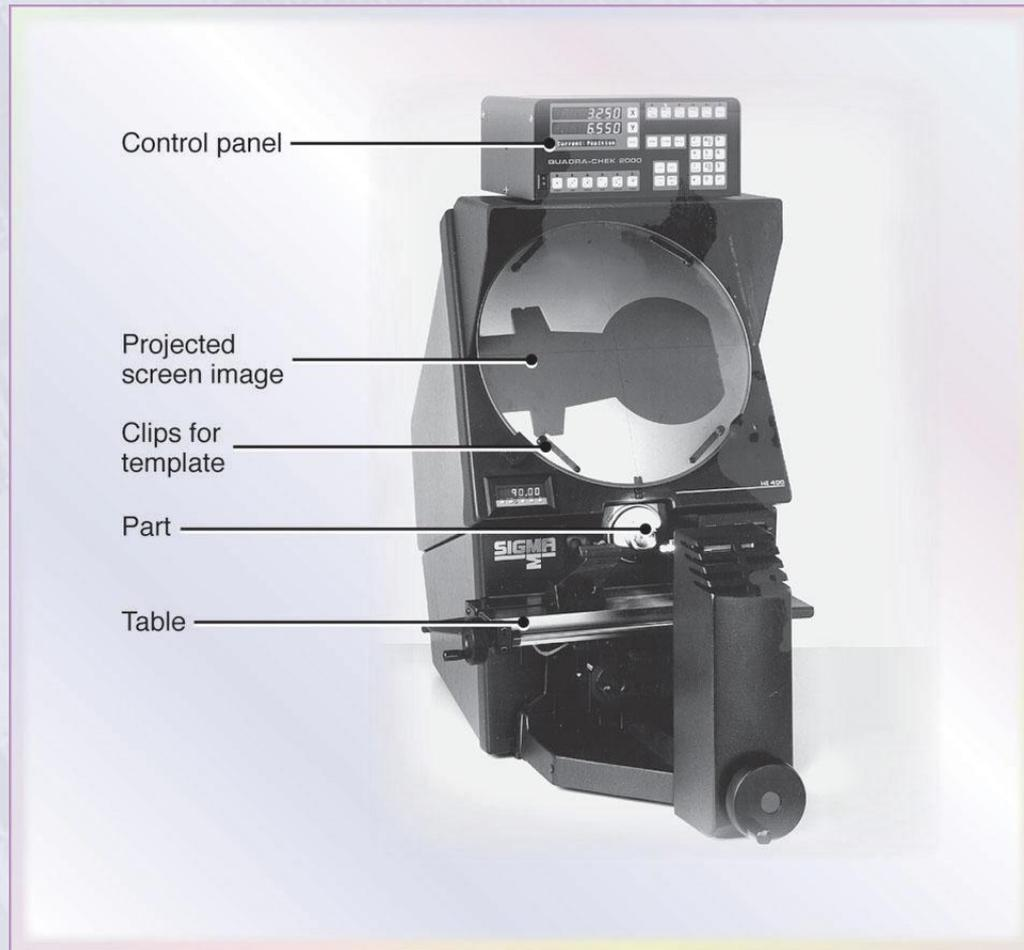
Figure 35.9 A bench-model horizontal-beam contour projector with a 16-in. diameter screen with 150-W tungsten halogen illumination. *Source:* Courtesy of L. S. Starrett Company, Precision Optical Division.
